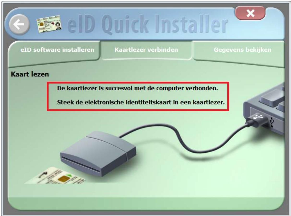
You will get a message saying “The card reader has successfully connected to the PC. Insert the electronic ID card into the reader”
