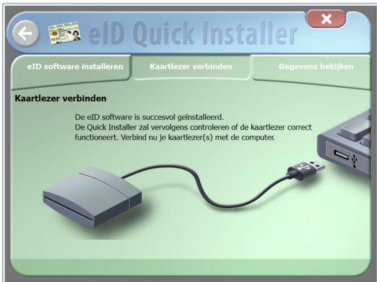
Connect the card reader to the USB port. Make sure it is empty and does not yet have an eID card inserted into it.
